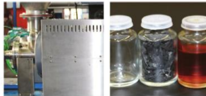
Lab unit with 2 kg/h feedstock capacity tested at Fraunhofer UMSICHT
